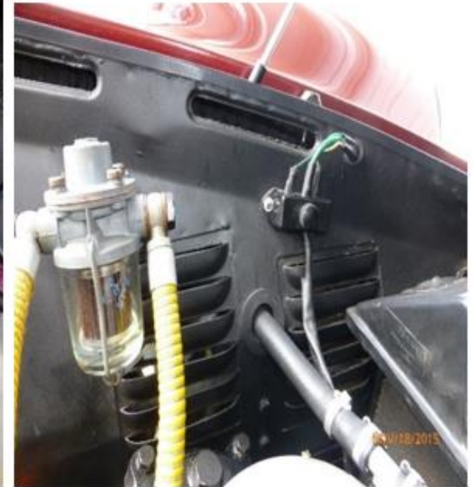
11) Alternator junction box
