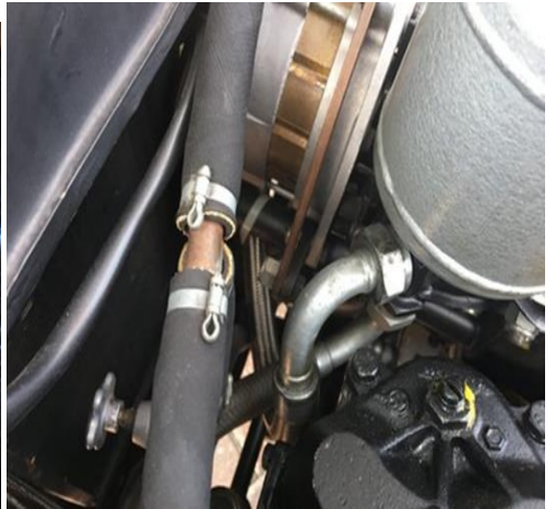
9) Water heater hose and Copiglia clamp
