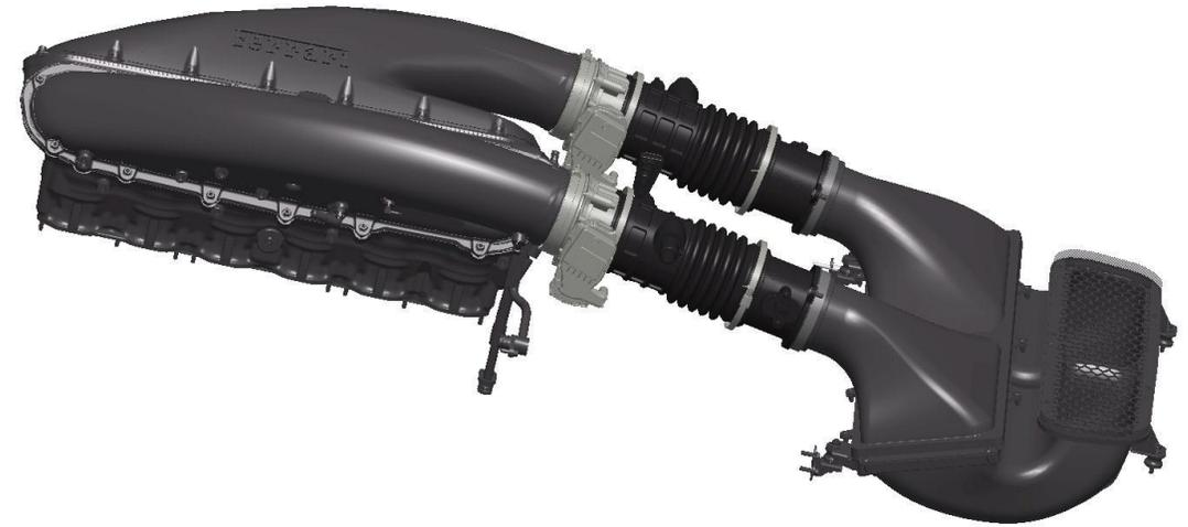
Fig. 4 - Intake assembly
