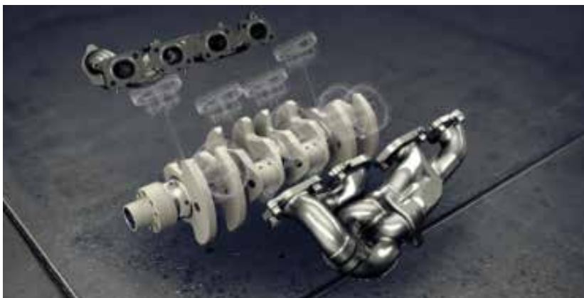
Flat-plane crankshaft and three-piece cast exhaust manifold and turbo housing
