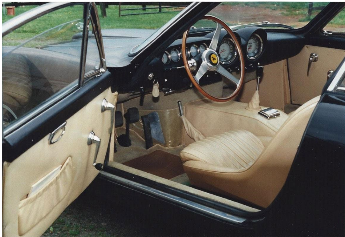
35. Original interior, pucker door pocket and console and plastic scuff guard. 250 Lusso. Image Greg Jones
