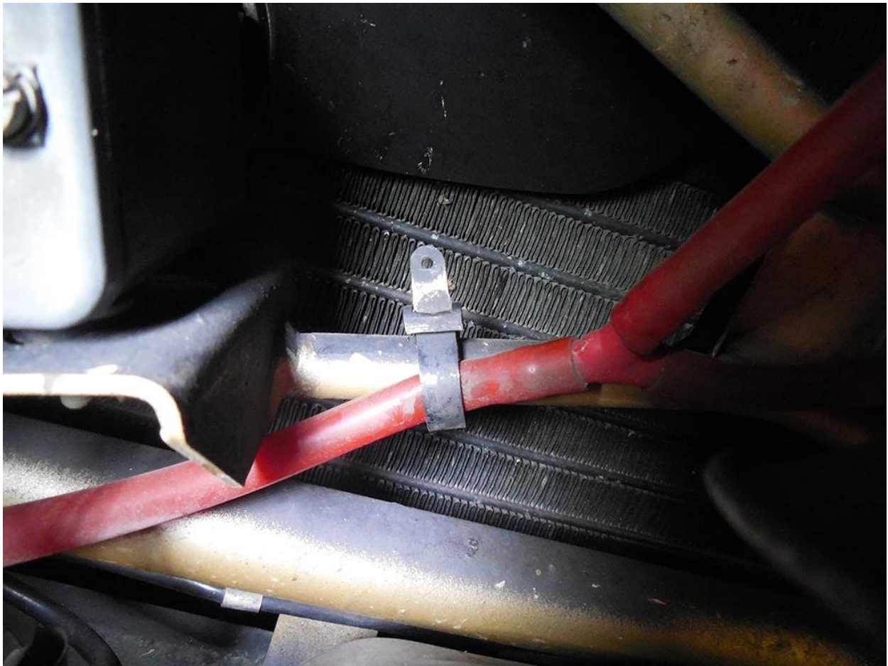
19. Black overspray on body-colored frame expected as inner fenders were likely sprayed from rear before radiator and engine were installed. 330 GTC. Image Tom Yang
