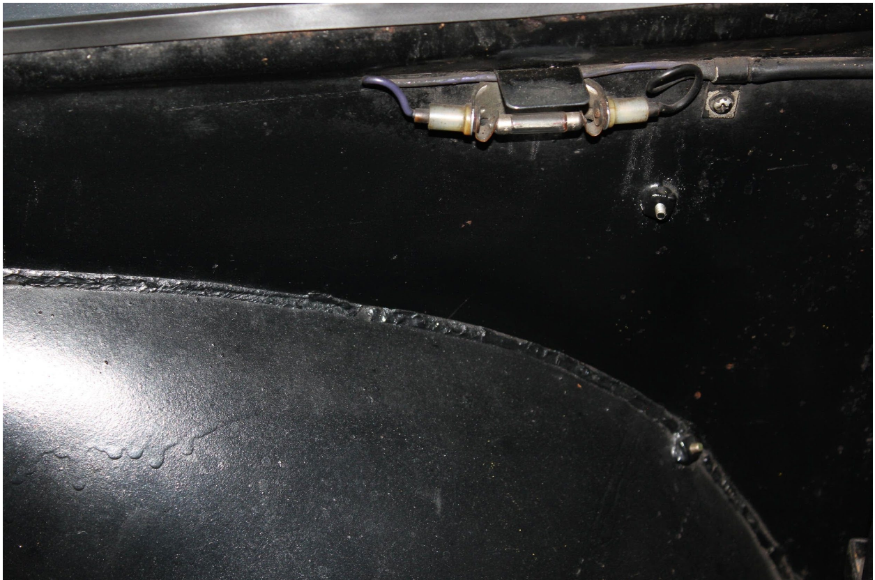
8. Hood latch originally painted over with welded latch and evidence of use. 250 Coupe. Image David Eichenbaum
