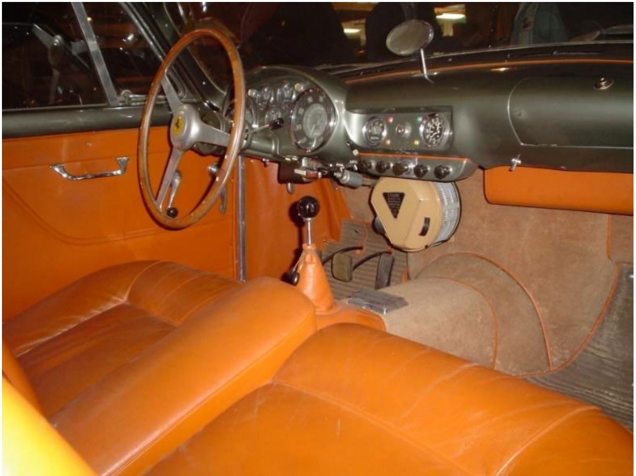
11. Original door skins, carpets, heel pads, piping, tassels, heater and dash. 250 Europa. Image David Carte
