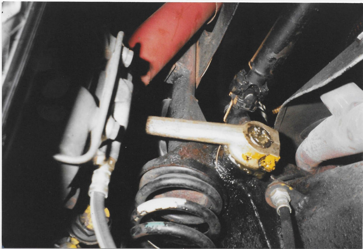
29. As-built suspension with yellow tightening marks intact. 250 Lusso. Image David Carte
