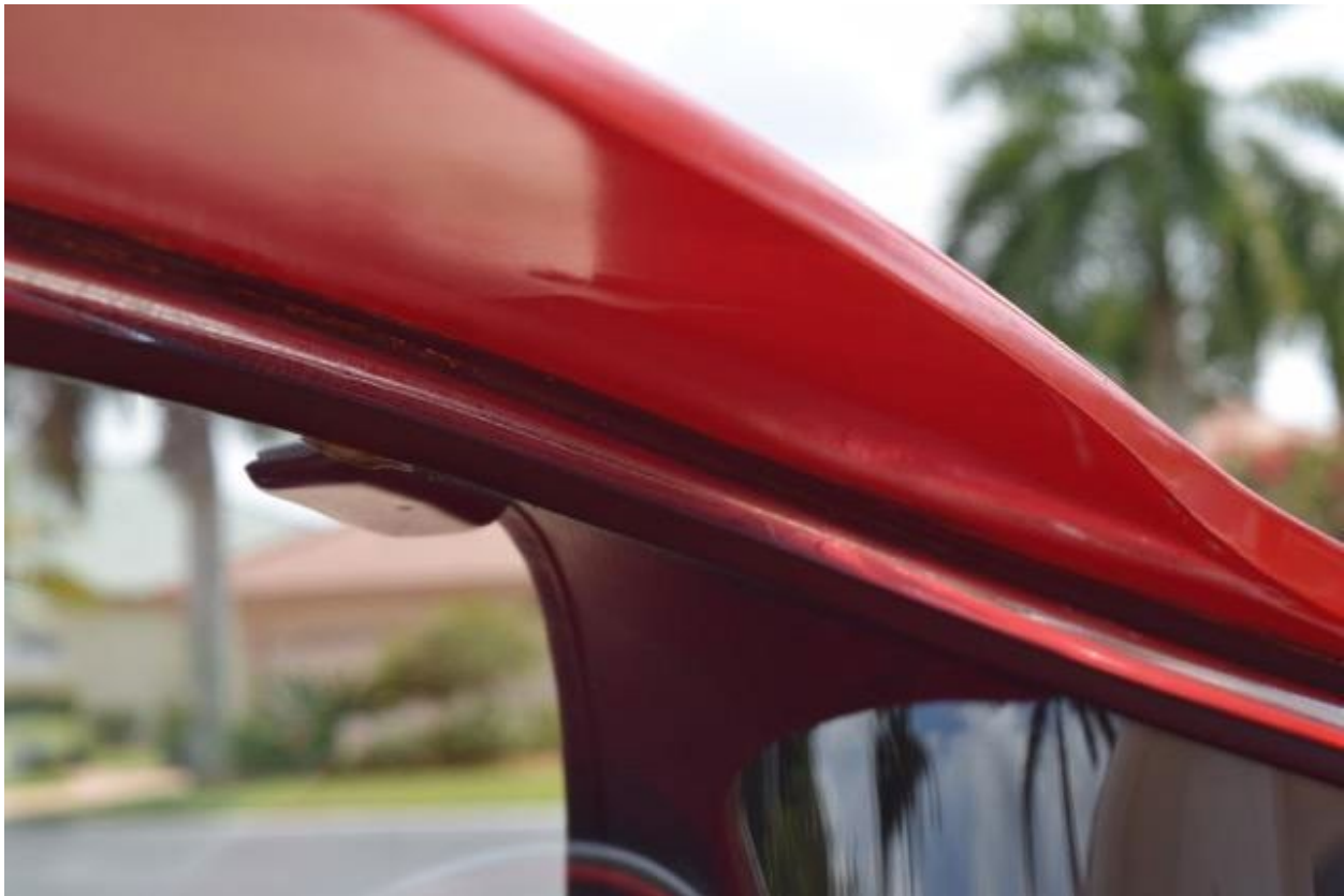
37. Typical factory paint blemish on door jam as delivered. 246 Dino. Image Marco Hartner
