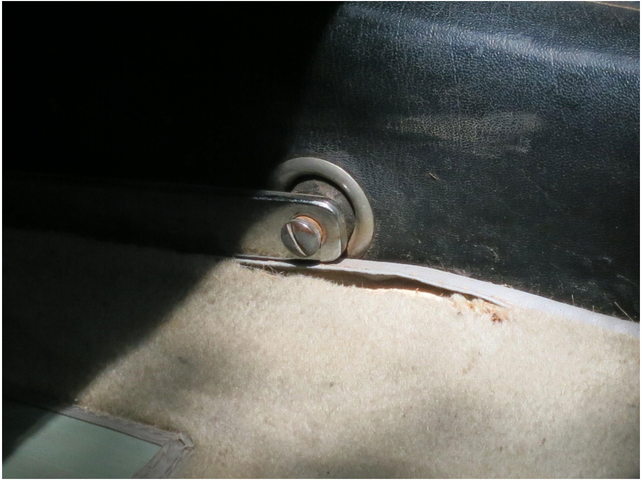
41. Note passenger footrest hardware, carpet weave, vinyl bound and stitched heel pad. 275 GTB Alloy. Image Donovan Leyden
