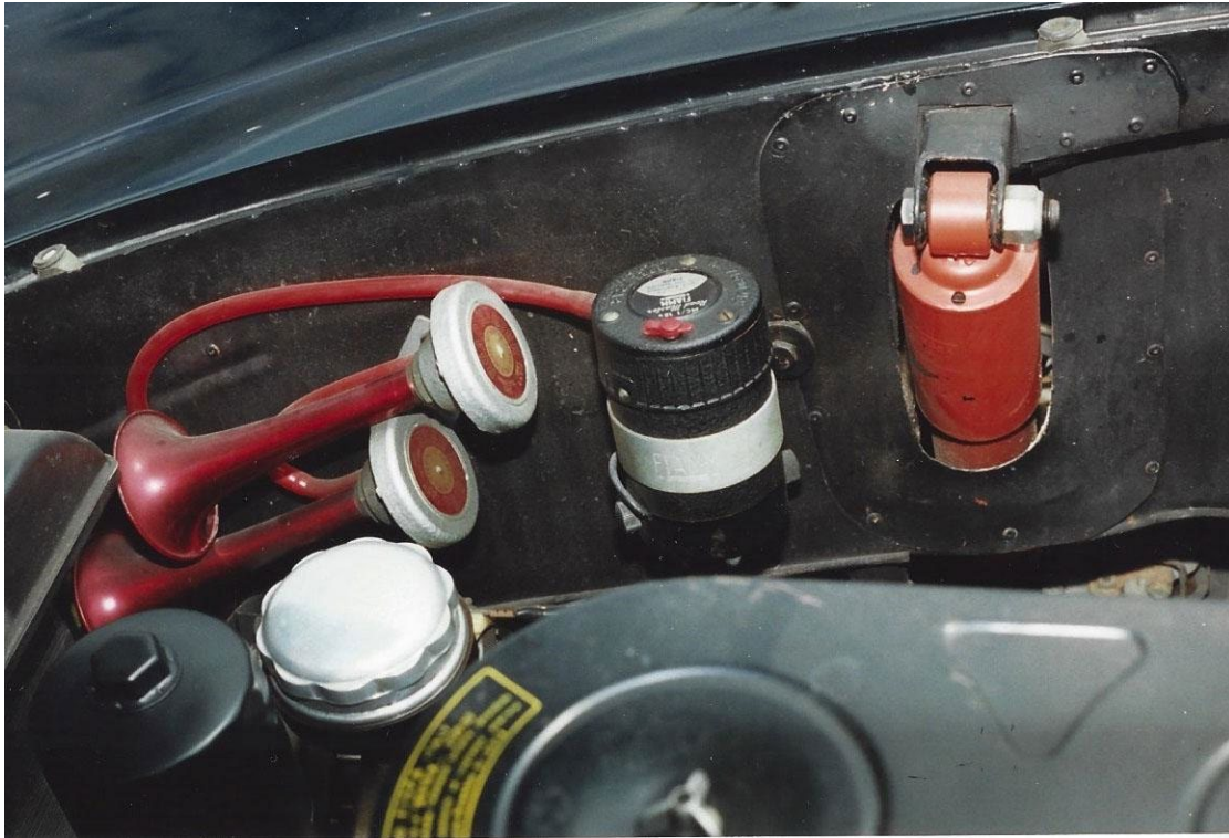
30. Typical original Lusso engine compartment except repainted oil filter. Note rivets, logos, horns. 250 Lusso. Image Greg Jones
