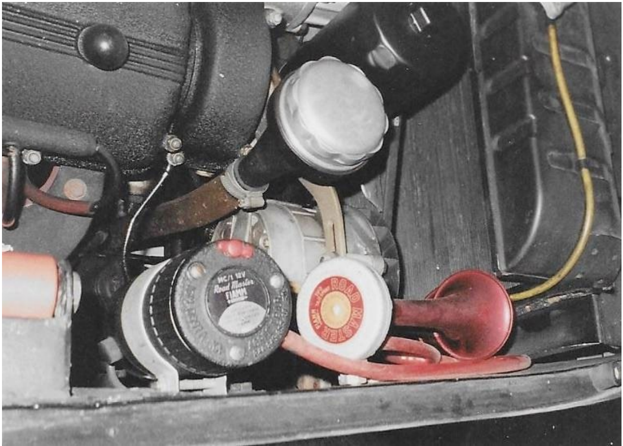
13. Typical unrestored engine details – except for painted filter. 250 GT Lusso. Image David Carte
