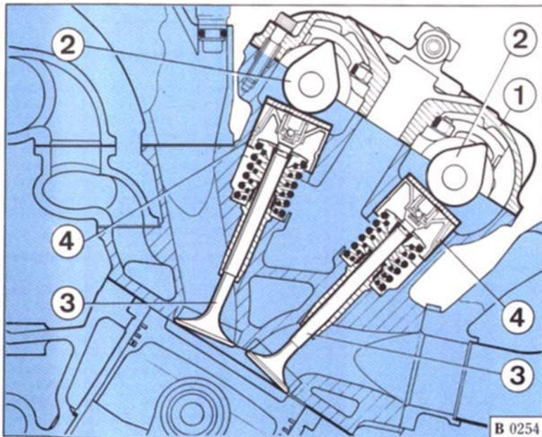
Valve timing features 4 head shafts (2 each cylinder bank) and 4 valves - two intake and two exhaust ones - each cylinder, driven by hydraulic tappets, having an automatic clearance recovery, thus keeping the same operating tolerance.
