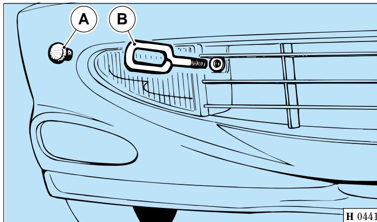
Remove the protective plug **A** and screw the eye-bolt **B** into the threaded hole.
