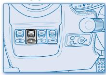
When the button is pressed, the rear fog lights are turned on only if the high beams or low beams are on. The dedicated warning light on the instrument panel comes on to indicate activation.
