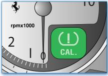
The system must be calibrated using the button on the dashboard after tyre replacement or inflation.
