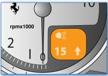
Briefly press the right-hand button **SET** to adjust the brightness of the instrument panel to a value between 0 and 30.
