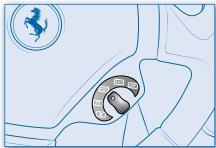
There are five modes available, which correspond to the grip level (from low to high) and consequently to the level of driving assistance required (from high to none).
