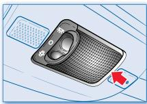
• Manually unclip the bulb holder pressing the two side locking tabs.
