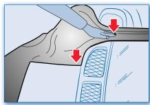
• Working in pair, stand on the two sides of the vehicle and, using both hands, first lift the rear end of the cover (1<sup>a</sup>) then push it (2<sup>a</sup>) and lift it towards the rear (3<sup>a</sup>), until it has reached the maximum opening position. The toolkit box, adequately protected, may be used to support the cover in this position if you do not have a suitable support.
