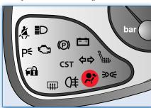
After activation, the pretensioners no longer function and they cannot be repaired under any circumstances. Contact the Ferrari Service Network to have them replaced.
