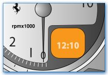
Briefly press the left-hand button MODE (less than 2 seconds) to sequentially switch between the various functions shown on the display:
