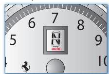
The system will automatically shift the gears UP and DOWN according to the vehicle speed, the engine RPM and the torque/
