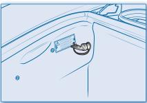
It is advisable to disconnect the battery if the vehicle is not used for long periods of time. Consult the section "If the vehicle is stored for long periods" in this chapter.
