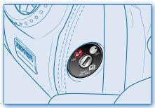
The LED remains on until the passenger airbag is reactivated.
