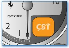
When the CST system is active, its operation is signalled by the relative warning light on the instrument panel and by the (green) message CST ACTIVE on the multi-function display, which flashes for at least 4 seconds.
